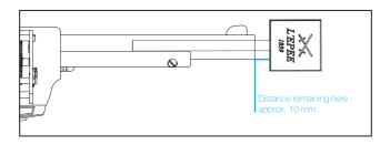
Make sure to wind up the spring completely. At the end of the winding procedure, you will feel the necessary force increase significantly; do not wind further as this is the sign that the movement is fully wound.
